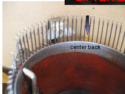
small gold knob at center back is the tension knob
