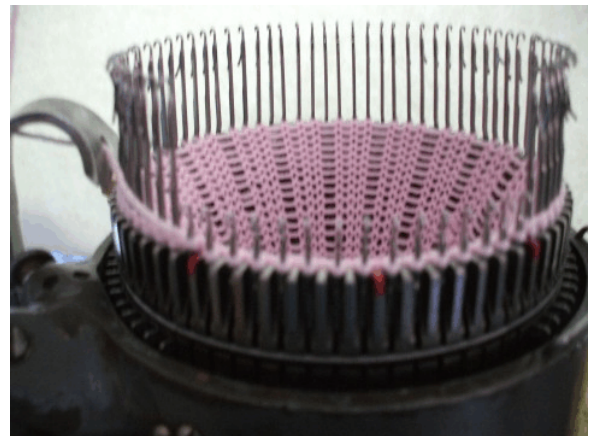
4. All but last left needle up; preparing to begin last decrease row
